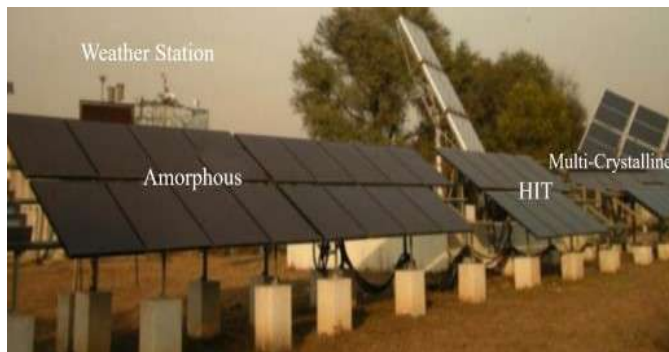
Fig.1 Outdoor test set up of three different PV technology modules at NISE, Gurgaon, India [23]
